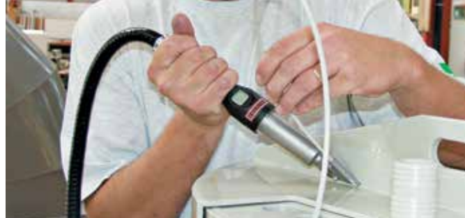
Draw welding using the compact and light Masa WELDING PEN R.
